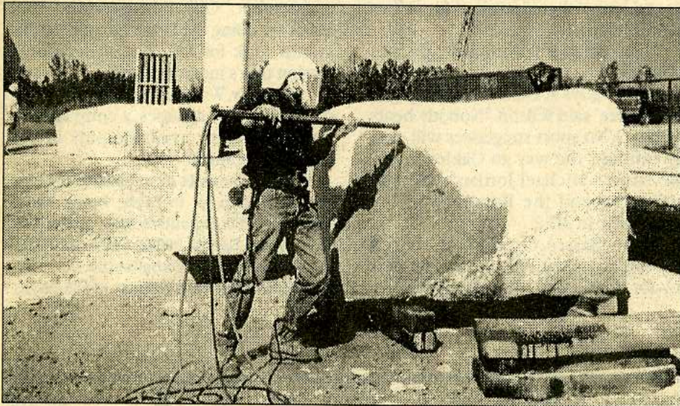
The stone is shaped with a touch that is usually used to burn channels in the ground so that granite may be quarried.
